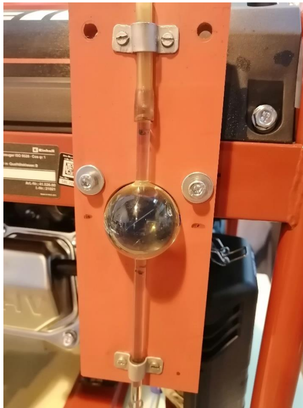
Metering bowl for measuring fuel consumption
