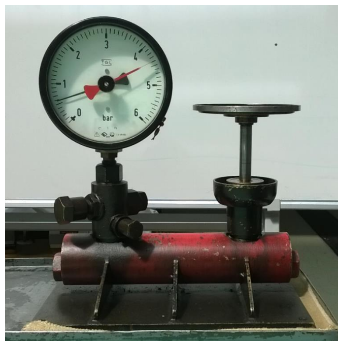
Figure 11. Apparatus used for calibration of manometer
