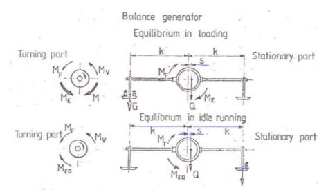
The <u>balance generator</u> is driven by the torque M. The equilibrium of the turning part (see Figure):
