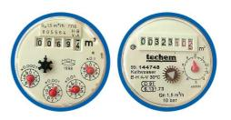
painted from 0-9 on the cylinder jacket we get the number of revolutions. Such a device is used in kilowatt-hour meters, water consumption, tape recorders, speedometers of cars etc.
