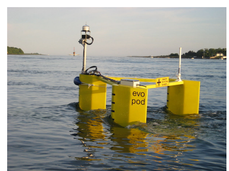
Evopod - A semi-submerged floating approach tested in Strangford Lough.
