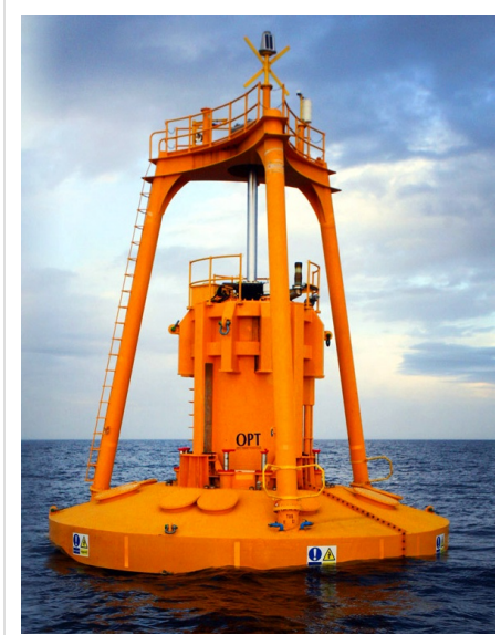
PB150 PowerBuoy with peak-rated power output of 150 kW.
