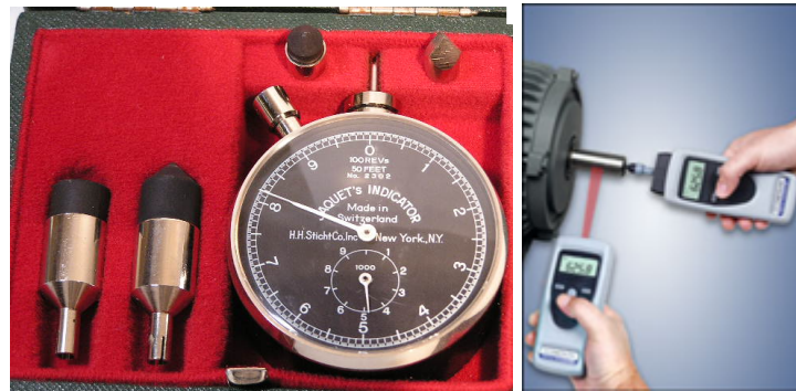
Figure 7: Left: Jaquet indicator. Right: Electric tachometer.
