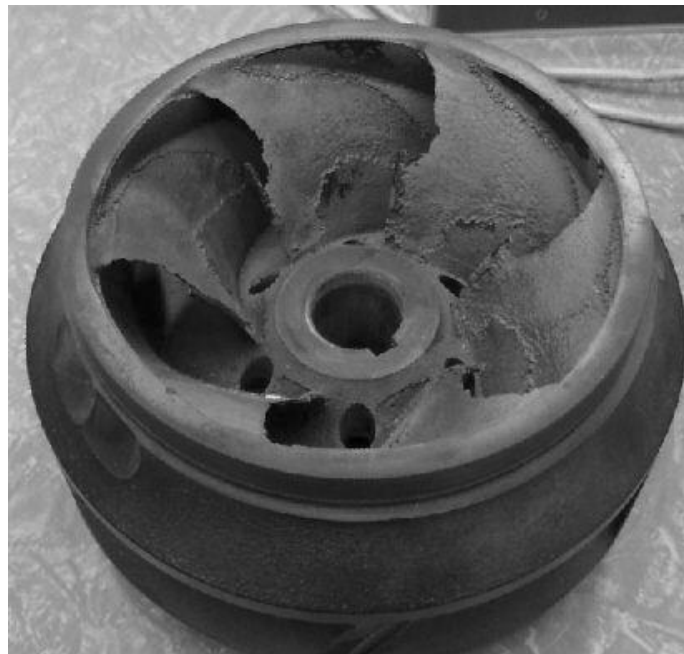
Figure 1. Signs of erosion because of cavitation on an impeller
