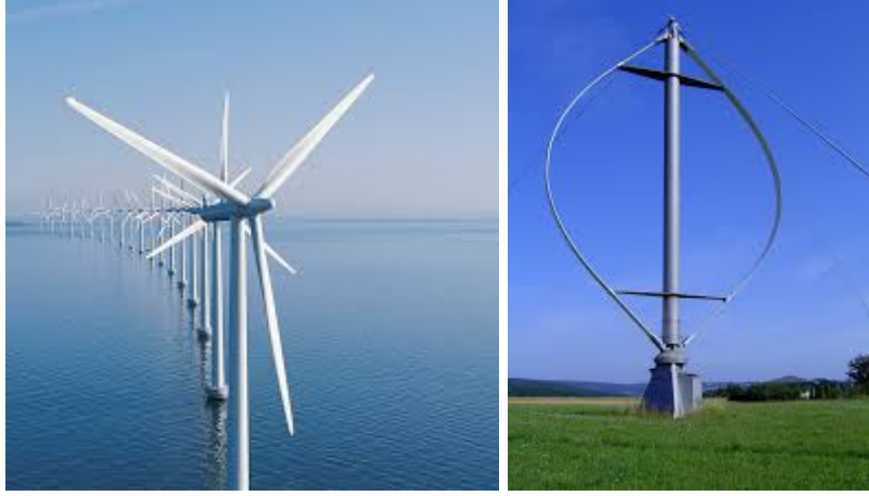
Figure 7.1: Typical examples of wind turbines. Left panel: horizontal axis wind turbine (HAWT). Right panel: Darrieus-type vertical axis wind turbine (VAWT).
