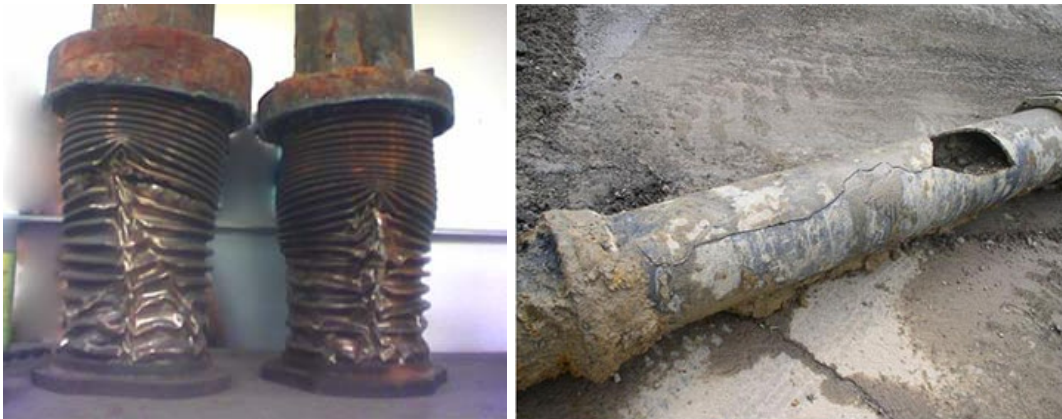
Figure 5.9: (Left) collapsed expansion joints due to depression wave. (Right) pipe burst due to chock wave (compression wave).
