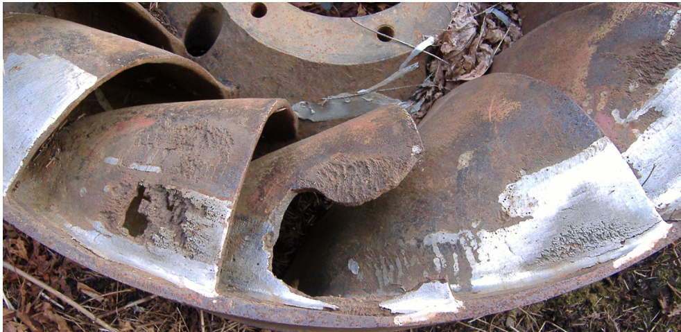
Figure 2.16: Illustration of the cavitation damage in pumps.
