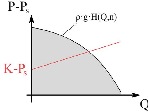
Figure 5: Graphical solution of the pump equation.
