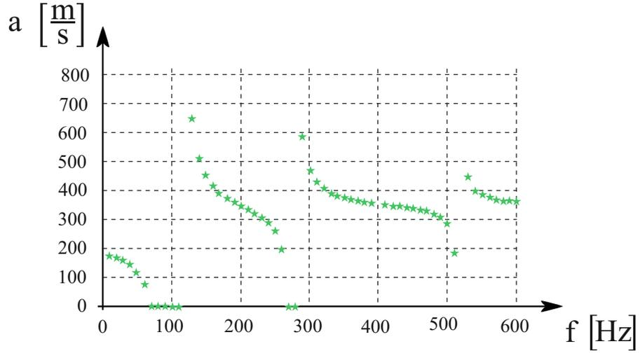
Figure 26: Wave velocity in a rectangular channel
