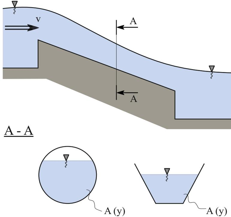
Figure 10: Open surface flow (schematic figure).
