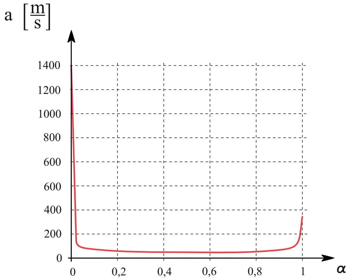
Figure 24: Wave speed in water containing air at 3 bar pressure
