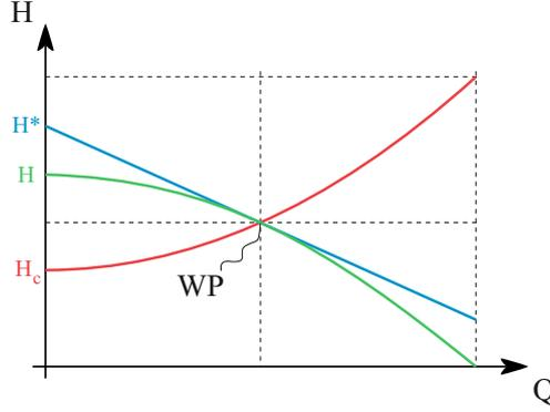
Figure 8: Pump characteristics.
